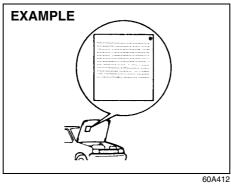
The EPA emission compliance label is located under the hood.
